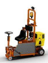
The Strassmayr S FF milling machines are used to prepare expansion joints or clean the cracks before application of special sealing compounds. Hydraulic drive of these compact and robust units allows easy and comfortable work. The steering wheel is directly connected with cutting tool, which allows smooth cutting regardless of the complexity of the course. Foldable protection of the operator and seatbelts secure the safety of the operator.
