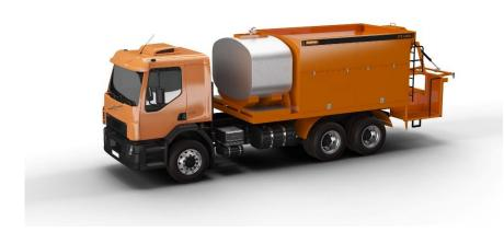
Strassmayr STR S is assembled on a frame or a 3 axle trailer and is designed to perform large road surface repairs using slurry seal and micro-surfacing technology.
